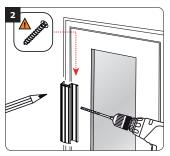
With the door closed, position the architectural handle onto the edge of the opening leaf of the door, ensuring the handle covers the box-section. Mark the vertical and horizontal holes, drill as required, then temporarily fix the handle leaving a small gap around the box section – check the alignment of the magnets in the handle.
