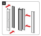
To finalise the assembly, tighten all fixings, and protect the handle fixing section by fitting the cover and end caps.
