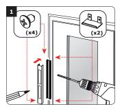
Position the box-section backplate, complete with pre-fitted electromagnetic locks, on to the door frame (or fixed door leaf if installing onto double doors) – ensure the positioning will allow for the archi-tectural handle to close securely over the section. Once you are satisfied with the position, mark the vertical and horizontal holes, then drill as required. Take note of the cable entry holes, and feed
